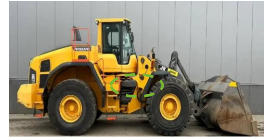
WLO battery installation
