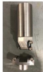
ILSS Test Fixture (ASTM D2344)
