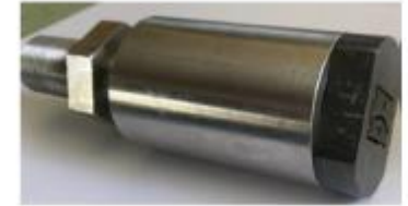
RCF Grip –shown here with curved wedge inserts for conduit tube fatigue testing for ITER
