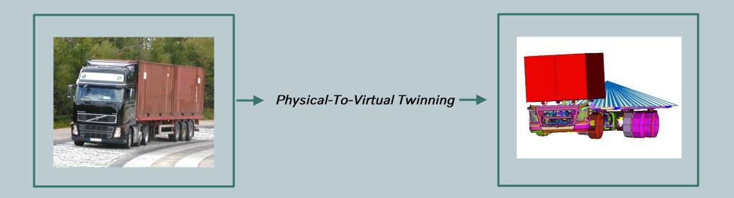
PURPOSE: Follow a test in real-time with a model (enhanced testing), estimate full stress and strain response in components during test (virtual sensing), etc.
