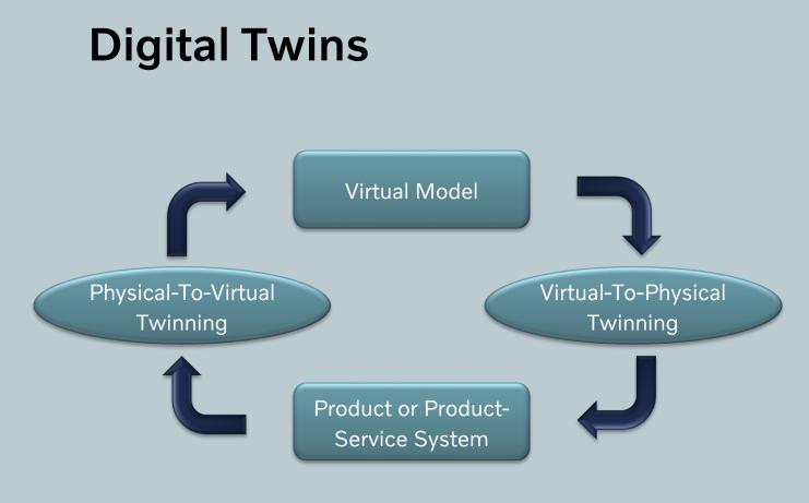
A digital twin is an integrated data-driven virtual representation of real-world entities and processes, with synchronized interaction at a specified frequency and fidelity.
