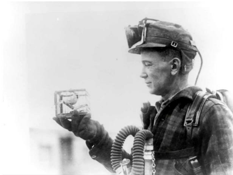
Mining foreman R. Thornburg shows a small cage with a canary used for testing carbon monoxide gas in 1928. (George McCaa, U.S. Bureau of Mines)
